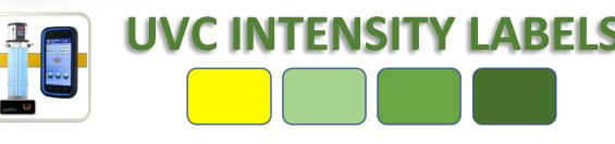
MRSA-UV's photochromic intensity labels are a basic, reliable, low cost, simple, inhouse method of monitoring specifically UVC intensity. When exposed to UVC light, the yellow labels undergo a gradual color change from yellow to dark green that is directly related to energy received.
